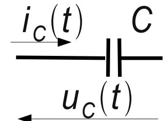
$$u_L(t) = \int \frac{I_C \sqrt{2}}{C} \cos(\omega \cdot t) dt = \frac{I_C \sqrt{2}}{C} \left[ \frac{\sin(\omega t)}{\omega} \right] + K = U_L \sqrt{2} \cos(\omega \cdot t + \varphi)$$
