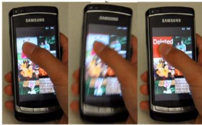
Fig. 4. Holding a photo (left) while shaking the device (middle) deletes the photo (right). Shaking again undoes the deletion.
