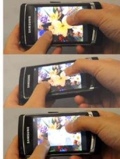
Fig. 3. Holding the screen with two thumbs (top) and then tipping the device away (middle) selects the indicated region (bottom).
