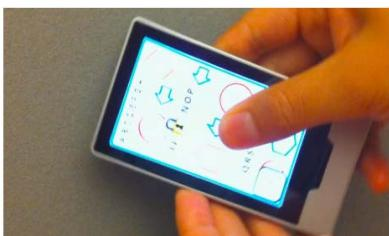
Fig. 2. Pivoting the device while holding the screen locks the current viewing orientation. A small padlock icon provides feedback.
