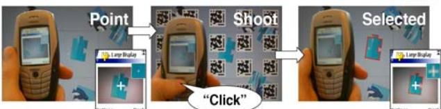
Figure 2. Point & shoot technique: (Left) The phone display is used to aim at a puzzle piece on a large display. (Middle) Pressing the joystick indicates selection and a visual code grid flashes on the large display to compute the target coordinates. (Right) The grid disappears and the targeted piece highlights to indicate successful selection.
