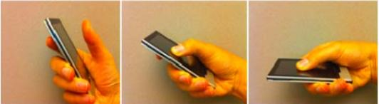
Fig. 1. Tilt-to-Zoom: No zooming occurs while the device is held normally (left). Touching the screen enters the zooming mode (middle). Zooming is then mapped to the change in tilt angle (right).
